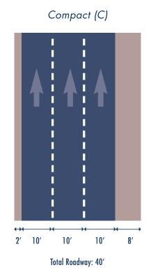
Expressway R: Expressway C: Regular Lanes **Narrow Lanes** and Shoulders and Shoulders **ROAD DESIGN PARAMETERS** 2 Number of Lanes 3 Lane Width (ft) 12 10 Left Shoulder Width (ft) 6 2 10 Right Shoulder Width (ft) 8 Total Roadway (ft) 40 40 Length (mi) 10 10 SPEED AND CAPACITY Free-Flow Speed (mi/h) 65.5 60.4 Speed at Capacity (mi/h) 52.3 51.2 Capacity per Lane (veh/h/ln) 2,114 2,068 4,228 6,204 Total Capacity (veh/h) TRAVEL TIME Free-Flow Travel Time (min) 9.2 9.9
